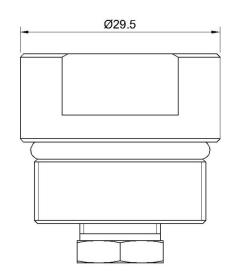
The C10 valve approved to EN ISO 17879 & ADR is a self-closing cylinder valve used for portable, refillable calibration gas cylinders.
