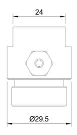
The C10 valve with Burst Disc is a self-closing cylinder valve used for portable, refillable calibration gas cylinders. This valve has a Burst Disc safety mechanism.
