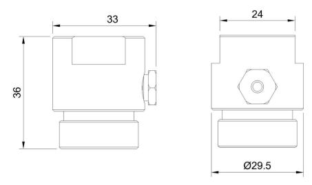
The C10 valve with Burst Disc is a self-closing cylinder valve used for portable, refillable calibration gas cylinders. This valve has a Burst Disc safety mechanism.
