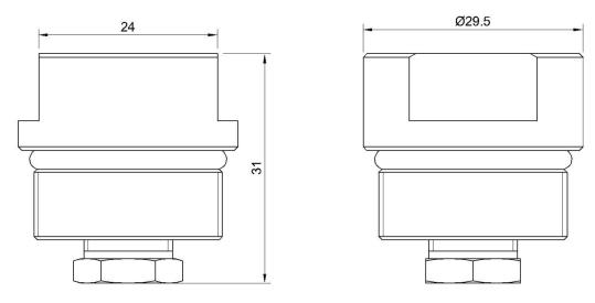
The C10 valve is a self-closing cylinder valve used for portable, refillable calibration gas cylinders.
