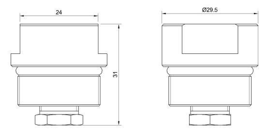
The C10 valve is a self-closing cylinder valve used for portable, refillable calibration gas cylinders.
