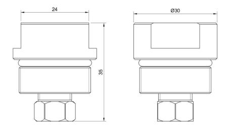
The non-refillable C10 valve is a self-closing cylinder valve used for portable, non-refillable calibration gas cylinders.
