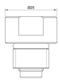
The C10 valve is a self-closing cylinder valve used for portable, refillable calibration gas cylinders.
