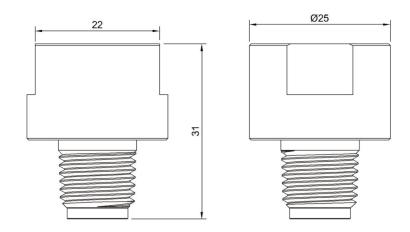
The C10 valve is a self-closing cylinder valve used for portable, refillable calibration gas cylinders.
