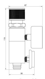
The 1210 regulators are adjustable two stage pressure reducing regulators. The two stage designs provides precise and stable outlet pressure as the inlet pressure reduces gradually
