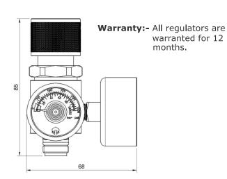
The 1250-M regulators are adjustable single stage pressure reducing regulators. These single stage designs provides stable outlet pressure irrespective to the reducing inlet pressure.
