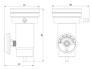
The CGA 600 Demand Flow Regulator is used for calibration gases, pump based instruments and handheld gas detectors. These regulators supply gas as demanded by the instrument and automatically shuts off.
