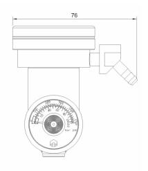
The Demand Flow Regulator is used for calibration gases, pump based instruments and handheld gas detectors. These regulators supply gas as demanded by the instrument and automatically shuts off.
