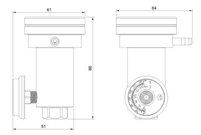
The High Pressure Demand Flow Regulator is used for calibration gases, pump based instruments and handheld gas detectors. These regulators supply gas as demanded by the instrument and automatically shuts off.
