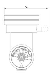
The Demand Flow Regulator is used for calibration gases, pump based instruments and handheld gas detectors. These regulators supply gas as demanded by the instrument and automatically shuts off.
