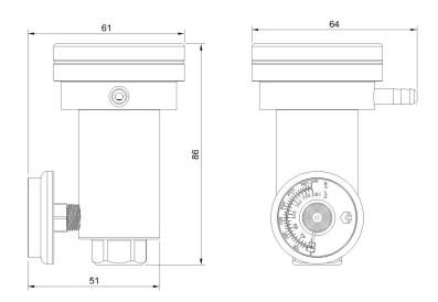
The High Pressure Demand Flow Regulator is used for calibration gases, pump based instruments and handheld gas detectors. These regulators supply gas as demanded by the instrument and automatically shuts off.
